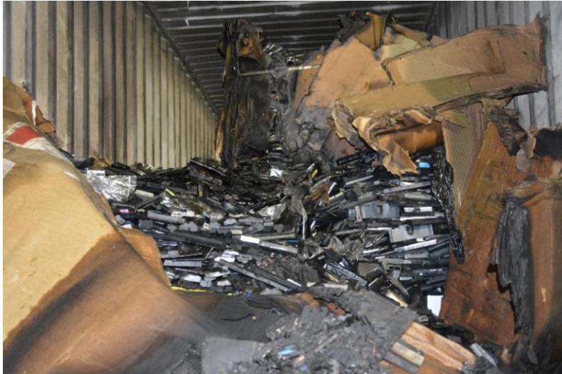
Burned lithium batteries in fiberboard boxes after the August 19, 2021 fire. Photo courtesy U.S. Coast Guard
