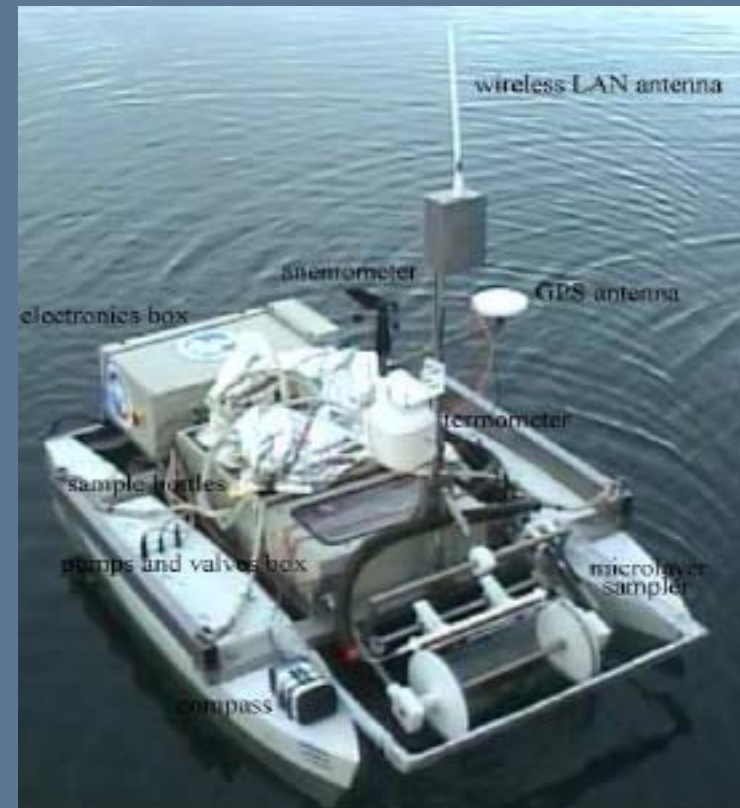
SESAMO (SEa Surface Autonomous MOdular unit) configuration by the Italian National Program of Research in Antarctica (PNRA), and carried out in cooperation with the CNR Institute for the Dynamics of Environmental Systems, Venice
