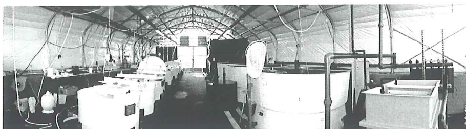
Figure 2 View of the eco-toxicological testing facilities of Cedre: on the left, the 14 tanks used to expose the animals to the pollutant, on the right the stabilization tanks
