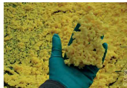
△ Crust of sulphur following a release of molten sulphur into Cedre's deepwater test tank
