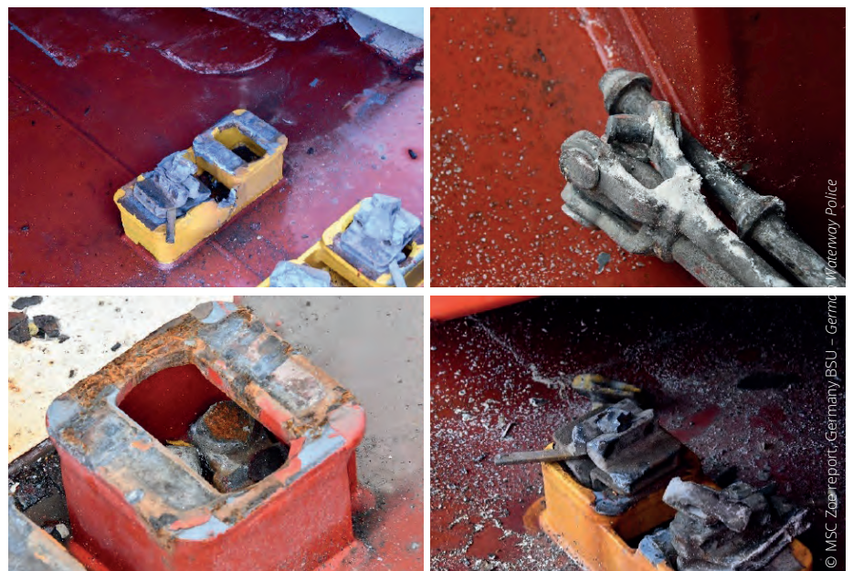
▲ Broken parts: deck fittings, twistlocks, turnbuckles
