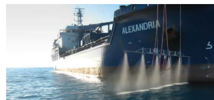
Starboard spraying arm of the Alexandria (Source: EMSA)
