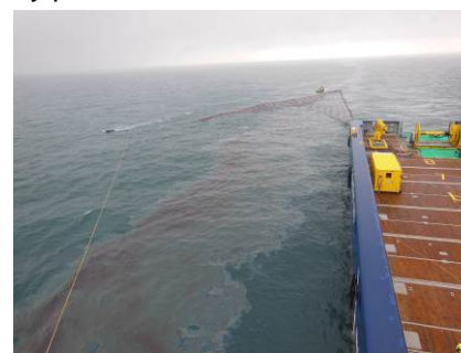
Deploying the MOSS Sweeper 50 from the Stril Luna (Source: NOFO)
