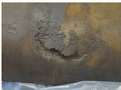
Left: Close-up of the breach in the line (Source: PHMSA); Right: Visible crude oil leak at a drainage culvert (University of California Santa Barbara)
