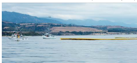
21/5/15: Pair trawling of floating booms off Santa Barbara (Source: USCG)
