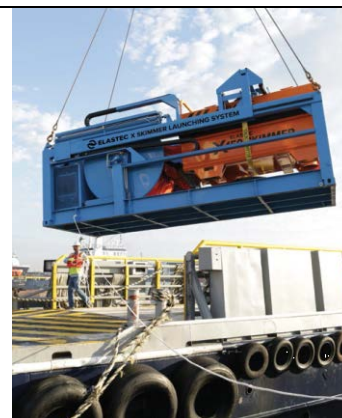
The X150 Skimmer Launching System being crane-lifted onto a vessel's deck (Source: Elastec)
