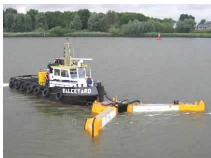
The Victory Oil Sweeper operated by a push-tug (Source: Koseq)
