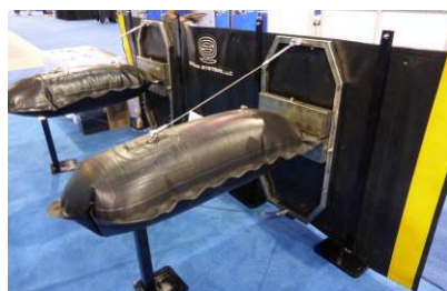
Left: The floats positioned on the outside of the ORS-1000's deflection boom arms (Source: Cedre); Right: The 2 rows of weirs concentrating the oil at the apex of the system (Source: Ocean Systems LLC)
