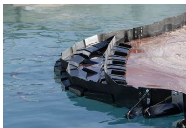
Left: The floats positioned on the outside of the ORS-1000's deflection boom arms (Source: Cedre); Right: The 2 rows of weirs concentrating the oil at the apex of the system (Source: Ocean Systems LLC)
