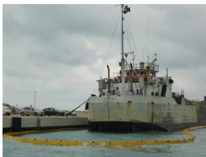
Containment booms around the Nijptangh , in dock for fuel removal (Source: Cedre)
