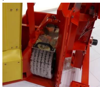
The rotating oleophilic brush skimmer at the base of the sweeping arm (Source: Cedre)
