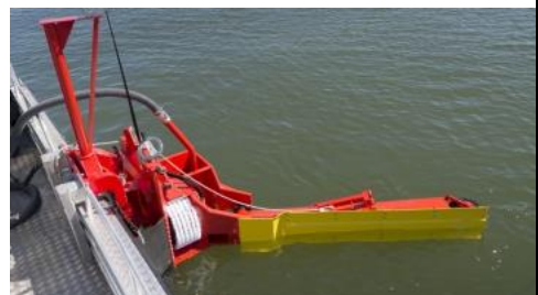
The MiniBagger sweeping arm (Source: SeaHow)
