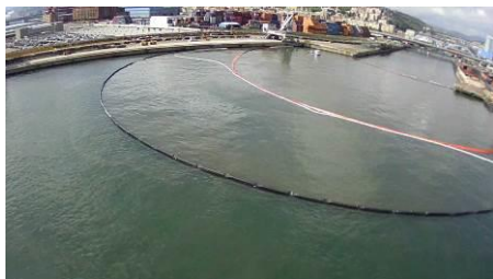
View from a Hawk Owl surveillance device deployed by Castalia: rows of booms across the Polcevera which feeds into the port of Genoa (Source: Castalia Consorzio Stabile S.C.p.A.)
