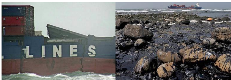
View of the structure of the TS Taipei, with a vertical breach on 25/03/2016; Heavy fuel oil washed up on the rocky foreshores some 300 m from the wreck (Source: Taiwan Environmental Protection Agency)
