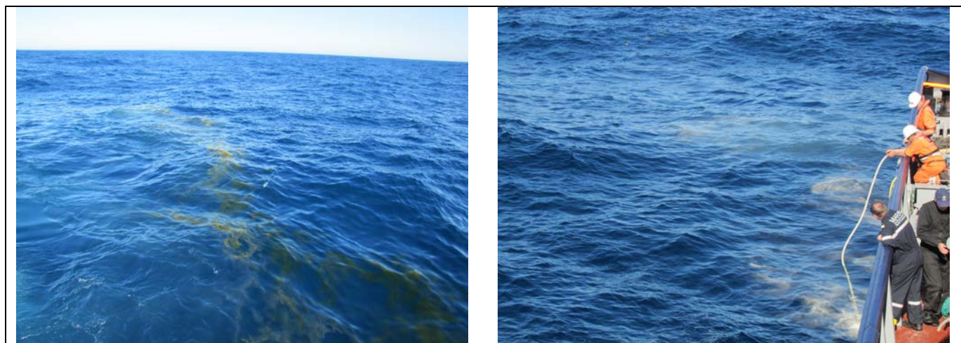
Figure 4 Third flight: rapeseed oil (left) and FAME (right) release from the boat.
