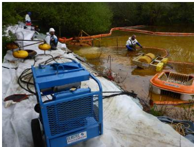
Area of natural accumulation of free pollutant (northern wall of second pond): deployment of oleophilic drum and disc skimmers (left); manually unclogging a Mini Foilex weir skimmer (centre) clogged with weathered biodiesel, amalgamated with plant debris (right); (Source: Cedre)
