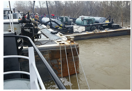
23/01/2016: Lightering operations on the tanker barge MM-46 (pumping and transfer to a barge brought alongside) (source: USCG)
