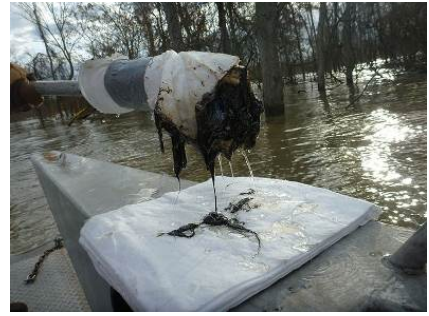
An effective "low-tech tool" for detecting sunken oil (Source: NOAA)
