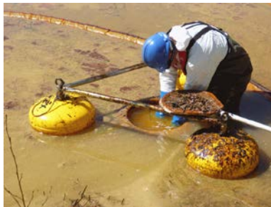
Area of natural accumulation of free pollutant (northern wall of second pond): deployment of oleophilic drum and disc skimmers (left); manually unclogging a Mini Foilex weir skimmer (centre) clogged with weathered biodiesel, amalgamated with plant debris (right); (Source: Cedre)
