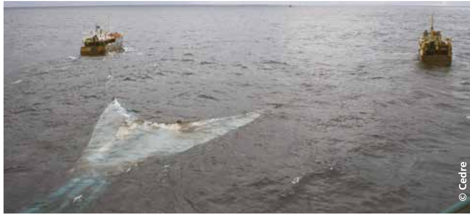
A Seynipp spill response trawl system being deployed by fishing boats
