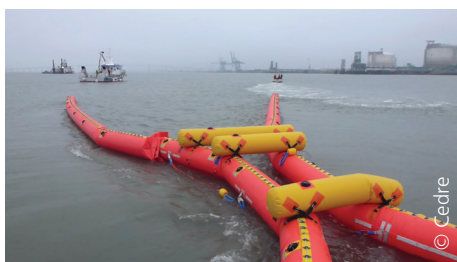
Operating the Current Buster 4 in dynamic mode with two boats
