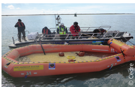
Skimming the simulated spill in the apex of the Current Buster 2 and transfer to the floating storage capacity
