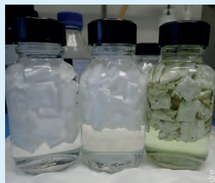
^ Studying the release of contaminants by new and weathered EPS on Cedre's artificial beach
