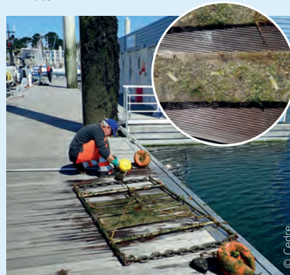
^ Underwater device used to study the breakdown of cigarette butts, installed at the Marina du Château in Brest, in collaboration with Brest's marinas
